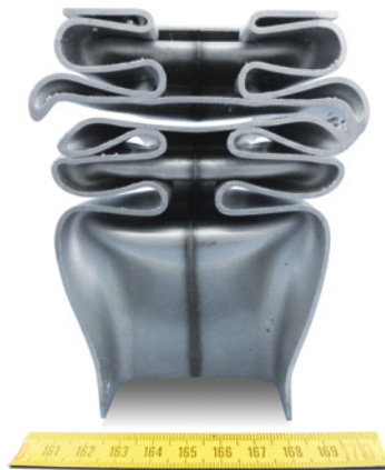
High ductility of MnCr materials in welded areas
